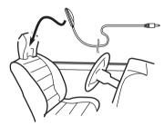
The auto TA and EQ may differ depending on where you place the microphone. If desired, place the microphone on the front passenger seat to perform auto TA and EQ.
