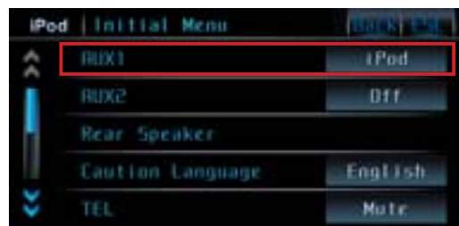
2. AUX 1 should be switched to "iPod" in the initial menu. The initial menu is available even if the source is off.
