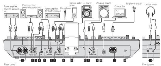
MASTER OUT 1 terminals Connect a power amplifier, powered speakers, etc., here. Be sure to use these as balanced outputs. Be careful not to accidentally insert the power cord of another unit.
