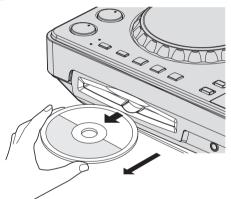
If the [DISC▲] button is pressed accidentally, press the [PLAY/PAUSE►/II] button immediately. Disc ejection is canceled and the unit is reset to as it was directly before the [DISC▲] button was pressed. (No sound is output during the resetting process.)
