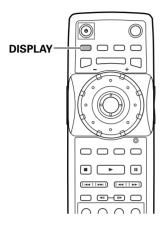
Press **DISPLAY** during while a disc is playing. Press **DISPLAY** repeatedly to change the information being displayed.
