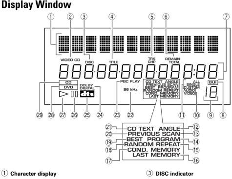
Displays text information already recorded on the disc such as CD TEXT or DVD text, and also text manually input into the player.
