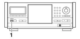
1 Press 🕁 STANDBY/ON on the front panel (🕁 on the remote control).
