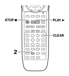
1 Play a disc that has a Last Memory point memorized and then press **STOP** ■ to stop playback.
