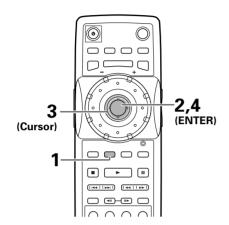
3 Move the cursor control joystick to select one of the preprogrammed picture quality settings. Standard\*: Preset that presents the source video as it is, with no special adjustments.
