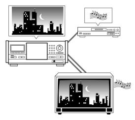
The input jacks on this player can be used for external audio and/or video input from a separate component. Additionally, when these kind of connections are made, it is possible to mix and match the audio and video inputs as you like.
