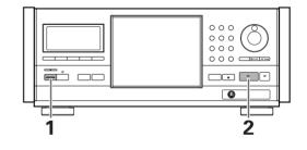
1 Press ひ (ひ STANDBY/ON on the front panel).
