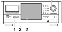
1 Press **SINGLE LOADER ACCESS** on the front panel.
