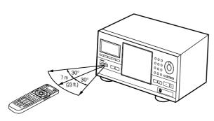
When operating the remote control, point it at the remote sensor (n) located on the player's front panel. The remote control can be used up to 7 m (23 feet) from the player and within a 30° angle on each side of the sensor.
