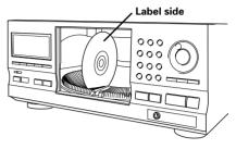
4 Press SELECT DISC NUMBER (the dial mode indicator lights green) and then turn MULTI DIAL to rotate the rack to the next position.
