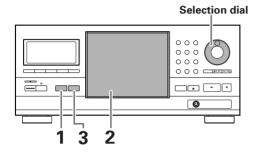
1 Press **SINGLE LOADER ACCESS** on the front panel.
