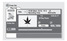
3 Use the playback controls (▶, II, ◄◄, ▶▶, etc.) to find the start of the section to erase, then (with 'From' highlighted) press ENTER.
