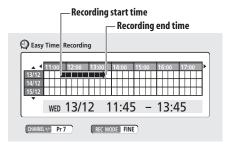
As you move the cursor around the grid, an arrow stretches from the start time to the current cursor position, representing the length of the recording. A recording of up to six hours can be set.
