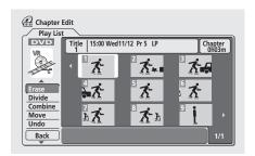
Erase – Erase chapters: Select the chapter you want to erase and press ENTER. • **Divide** – Divide a chapter into two or more parts: Select the chapter you want to divide. From the following screen use the playback controls (▶, Ⅱ, ◄◄, ▶►, etc.) to find the point at which you want to divide the chapter. With **Divide** highlighted, press **ENTER**.
