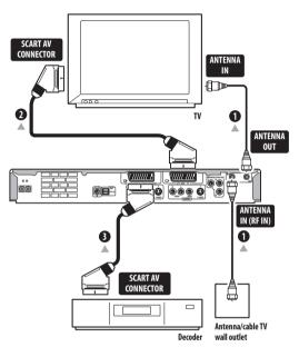
1 Connect RF antenna cables as shown.
