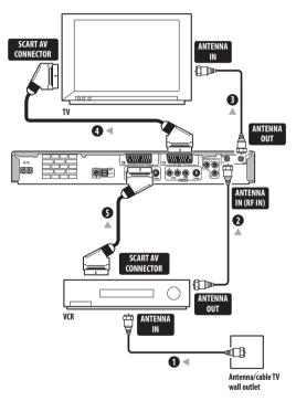
1 Connect the cable from the antenna/cable TV outlet to the antenna input on your VCR.
