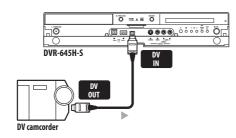
• Use a DV cable (not supplied) to connect the DV jack of your DV camcorder/video deck to the front panel DV IN jack of this recorder.
