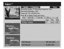
Select from **AUTO**<sup>1</sup>, **FINE**, **SP**, **LP**, **EP**, **SLP**, or **MN** (if manual recording is set to **On**.)
