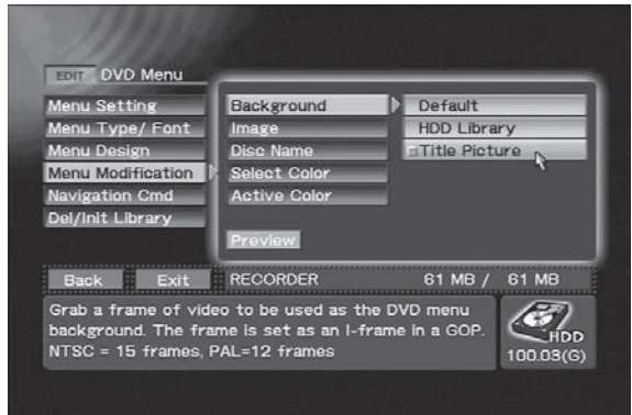
Using EDIT section → [DVD Menu] → [Menu Modification] → [Background] to select Title Picture
