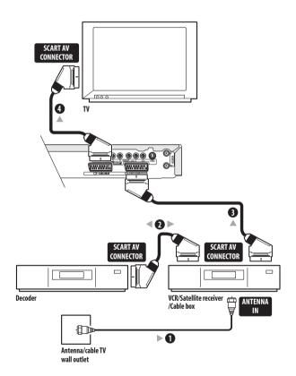
1 Connect the cable from the antenna/cable TV wall outlet to the antenna input on your VCR/ satellite receiver/cable box.
