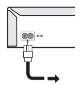
1 Plug the supplied AC power cable into the AC IN inlet and the other end into a standard household power outlet.
