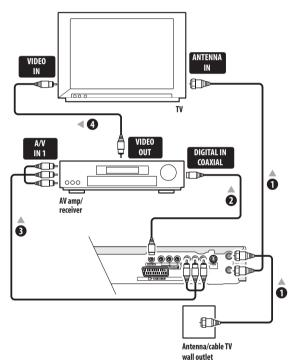
**1 Connect RF antenna cables as shown.** This enables you to watch and record TV channels.
