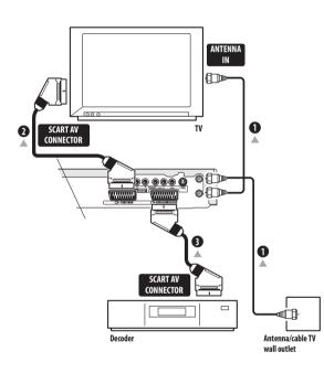
1 Connect RF antenna cables as shown.
