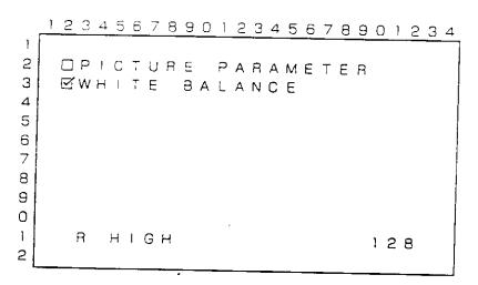
When operating from the remote control unit, perform the adjustment with the ◄ and ► buttons. When operating from the control panel of the Display, perform the adjustment with the + and − buttons. The adjustable range is 000 to 255. The value set on this screen becomes the center adjust value in the MENU mode.
