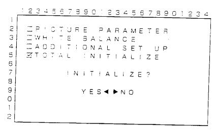
This function resets values adjusted for the Picture Parameters and White Balance back to the factory defaults. Note that this is limited to the data present in the memory area which is currently selected. Select Yes with the doubton on the remote control unit or with the + button on the control panel of the Display to default to the factory set values. Select No with the button on the remote control unit or with the button on the control panel of the Display to reproduce the current state.
