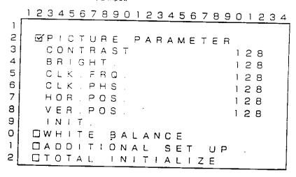
This mode is set when you press the MENU button in the standby state followed by pressing the Power button within 3 seconds. When operating from the remote control unit, select an adjust item with the ▲ and ♥ buttons and confirm your selection with the SET button. When operating from the control panel of the Display, select an adjust item with the + and − buttons and confirm the item with the SET button.
