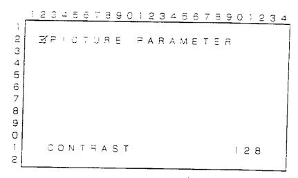
Use the ◄ and ► buttons to adjust from the remote control unit. Use the + and – buttons to adjust from the control panel of the Display. The adjustable range is 000 to 255. The value set on this screen becomes the center adjust value in the MENU mode.
