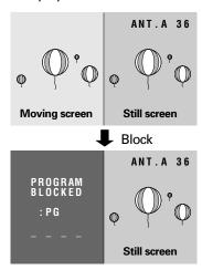
When blocking is on during SEARCH screen mode, the screen at search picture side will be blacked out (mute) without displaying: "PROGRAM BLOCKED".
