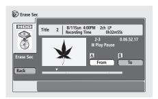
3 Use the playback controls to find the start of the section to erase, then (with 'From' highlighted) press ENTER
