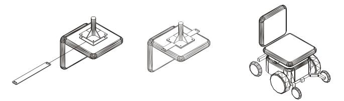
**Anchor U-Bolts:** The U-Bolts are to be used with Power Chairs or Scooters that do not have a center seat post. On this type of chair, the seat is normally attached to a tubular frame. Attach the U-Bolts, two on each side, to the frame as shown below. Make sure that the loop extends to the outside of the chair to allow the strap hooks to be attached by the end user.
