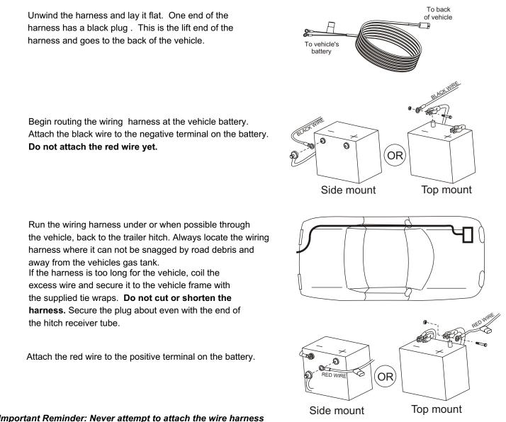
Important Reminder: Never attempt to attach the wire harness to a secondary power source, The lift requires direct connection to the battery.
