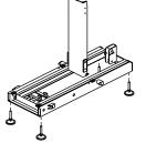
**Placing the lift into the vehicle:** Pick up the lift and place it into the vehicle's cargo area. This operation will require two people to perform. Take care during this operation not to scratch the vehicle's interior. Position the lift such that it will be one inch inside of the rear door. Verify this by closing the rear door and inspecting the fit from inside of the vehicle.
