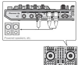
To output the sound from the [BOOTH] output terminals, connect devices such as speakers to the [BOOTH] output terminals.
