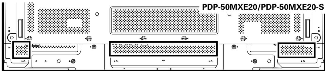
Connect the speed clamps using the 4 holes marked with "O" below, depending on the situation.
