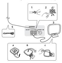
1 Pull off the protective shields of both AM antenna wires.
