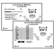
The configuration shown on-screen should reflect the actual speakers you have.
