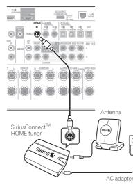
You will also need to connect the antenna and AC adapter to the SiriusConnect<sup>™</sup> tuner.
