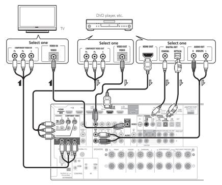
• Connect using an HDMI cable to listen to HD audio on the receiver. Do not use an HDMI cable to input video signals.
