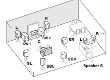
With these connections you can simultaneously enjoy 5.2-channel surround sound in the main zone with stereo playback of the same sound on the B speakers. The same connections also allow for 7.2-channel surround sound in the main zone when not using the B speakers.
