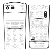
1 Point the remote control at the IR receiver and press  $\circlearrowright$  RECEIVER.
