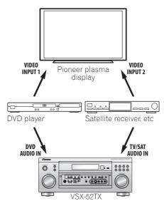
To make the most of the SR+ features, you should connect your source components (DVD player, etc.) in a slightly different way to that described in this chapter. For each component, connect the video output directly to the plasma display, and just connect the audio (analog and/ or digital) to this receiver.
