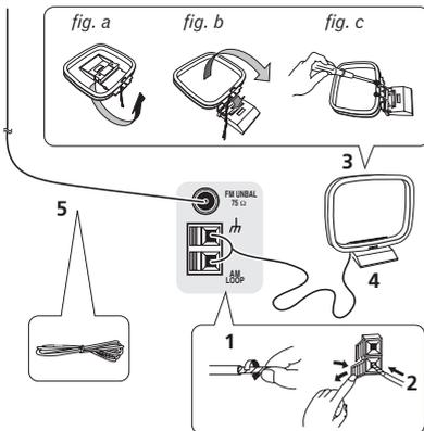
**1 Pull off the protective shields of both AM antenna wires.**
