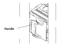
Shown above is the insertion to the front magazine bay. Though the insertion to the rear magazine bay is almost same but note that the proper installation position is in the place where it is very secluded.
