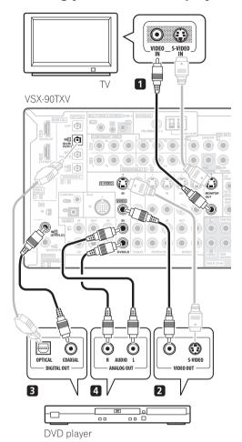
The diagram shows a basic setup of this receiver together with a TV and DVD player, with S-video or composite video connections. Different TVs and DVD players may offer alternative connections. See also *Using the component video jacks* on page 14 if your TV and/or DVD player has component video inputs/outputs. If your DVD player offers multichannel analog audio outputs, see *Connecting the multichannel analog inputs* on page 48.
