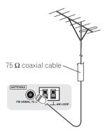
To improve AM reception, connect a 5 m to 6 m (15 ft. to 18 ft.) length of vinyl-coated wire to the **AM LOOP** terminals without disconnecting the supplied AM loop antenna.
