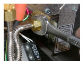
f. Install the orifice retainer bracket onto the pilot bracket and SCBS Orifice assembly. This will secure the orifice assembly into the runner tube.
