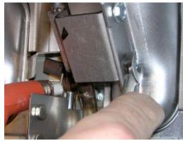
The SCBS Arm should now be mounted properly and securely. Inspect your work to insure that the burners are installed correctly. Improperly mounted or poorly aligned burners may result in an unsafe condition or poor appliance performance. They should be mounted properly on the orifice fittings, facing straight into the burner tubes and secured tightly to the appliance.
