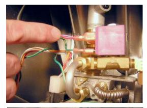
j. Route the SCBS Harness along the main control harness and wire tie it to the control harness. The proper wire tie locations are indicated by arrows, see photo at right. Trim excess from wire ties.
