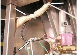
k. Mount the Thermal Limit Switch Assembly with the flange of the bracket oriented down and facing inward toward the tank. The switch terminals will then be facing outward toward the front of the appliance. Mount the assembly by straddling it on the two burners on either side of the pilot and positioned up to where the flange on the assembly meets with the bottom of the flange on the burner "web", see photos at right.
