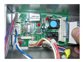
i. Connect the SCBS Harness to the SCBS Valve as shown. The red and violet wires must be connected to the vertically oriented tabs on the valve and the green (ground) wire must be connected to the bottom, horizontally oriented tab on the valve. The grey wires will be connected to the Thermal Limit at a later point in the upgrade process.
