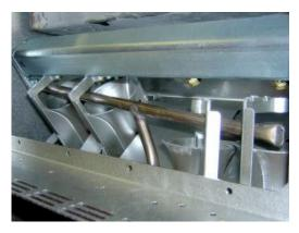
j. Secure the SCBS Arm to left side of the burner to the right of the pilot using two 10 X 24 self-threading screws provided with the Pitco Self-Cleaning Burner System Upgrade Kit.
