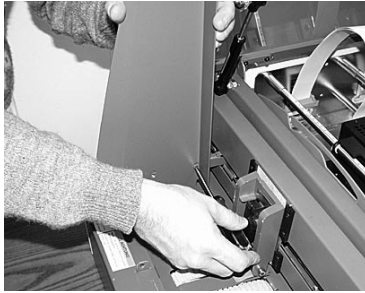
Installing the left side guide
