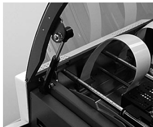
Properly installed shock
