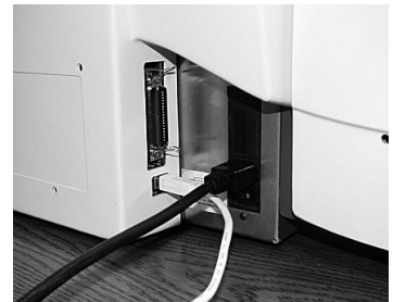
USB cable and power cord connections
