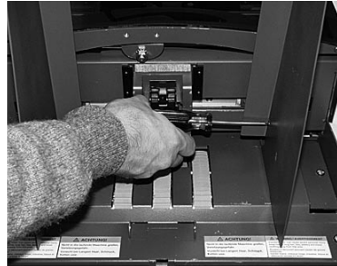
Installing the right side guide
