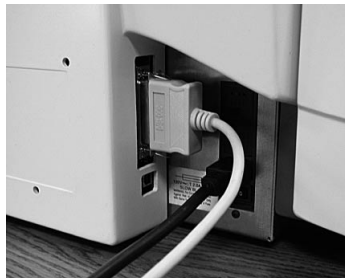
Parallel cable and power cord connections
