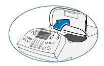
Close the cover. The system will automatically recognize the new cartridge, perform a brief maintenance operation, and return you to the home screen.
