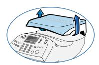
Flip open the ink cartridge cover. Lift and remove the old ink cartridge.
