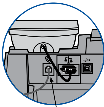
Plug phone line in here
