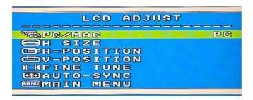
**PC/MAC** Switches between PC at 800X600 resolution and MAC at 832X624 resolution. Select PC/MAC, using [+] or [–] button. Then press [Menu] to initiate the switch between PC and MAC shown as above. Note: This function is to support MAC 832 x 624 resolution only.
