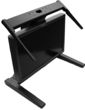
Bottom monitor assembly with mirror support arms and mirror adjustment screws
