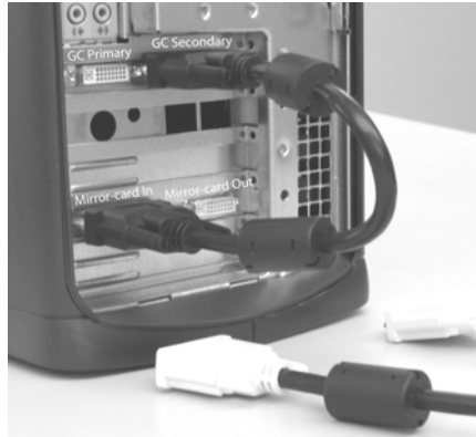
Short DVI cable installed.
