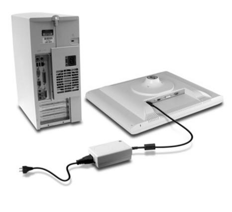
**2** Plug the power connector into the locking mini DIN port on the back panel.
