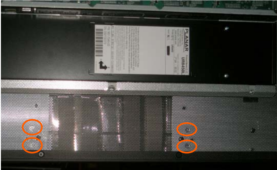
Landscape holes for kickstand bracket installation
