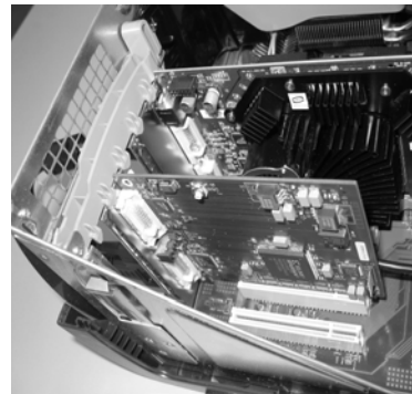
Mirror-flip PCI card installed
