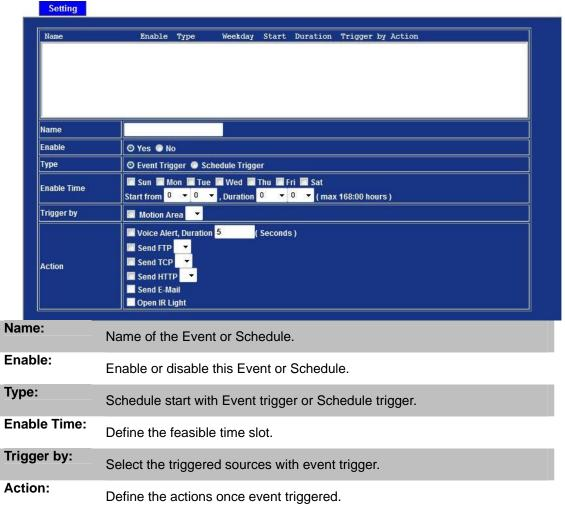
**Example1.** If you want to IR LED auto start in 18:00 every day and IR LED shines for 12 hours continuously. You will need to configure some parameters as below:
