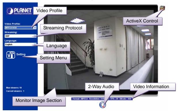
**Monitor Image Section:** The image shot by the IR IP Camera is shown here. The date and time are displayed at the top of the window.
