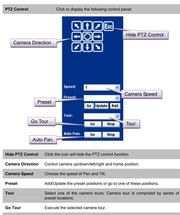
Auto Pan Execute the auto pan of camera. While auto pan is running, the camera will swing the camera automatically. Note that the speed of auto pan is fixed and cannot be adjustable.
