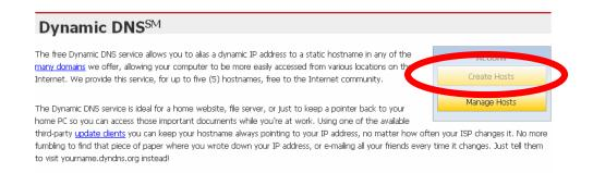
(11). We could create a domain name without any charge at this step. First, we input the host name. (No.1) Then we pick a domain that is easy to remember. Finally (No.2), click the "Add Host" to submit the domain name information. (No.3)
