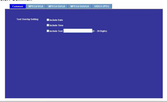
**Text Overlay Setting** There are some important information can be embedded into image, including date, time, and/or text.
