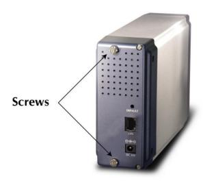
2. Grabbing the front panel and separate the HD holder from case.
