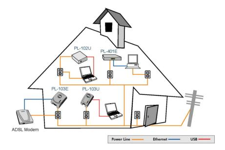
All the powerline devices on the network must use the same password to communicate each other. This password can be configured through the Powerline Configuration utility that can be found in the CD-ROM. The default password of PLANET powerline devices is "HomePlug". Thus, all the PLANET powerline devices can communicate each other without prior password configuration. Please refer to chapter 5 on detail of installing and using Powerline Configuration utility.
