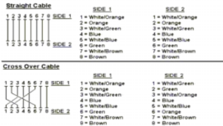
Figure A-1: Straight-Through and Crossover Cable
