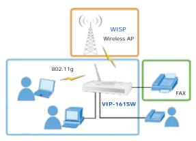
VIP-161SW Wireless Analog Telephone Adapter (1 x WAN, 1 x LAN, 2 x FXS)
