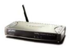
The WAP-4033 supports both IEEE 802.11b and IEEE 802.11g standards. You can use it for connecting to an existing WLAN, or to build up a new wireless LAN. Except essential AP mode, the WAP-4033 provides Repeater, Bridge, WDS, and Client modes to accommodate all kinds of network topology. High data rate (up to 54Mbps) performing allows faster communication between LAN and WLAN. Maximize network efficiency via using the WAP-4033 while minimizing your network investment and maintenance costs.
