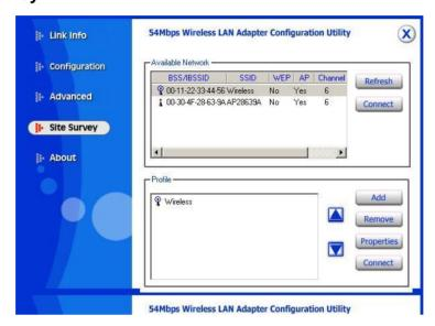
This screen shows the APs or Adapters which available fro WL-3560 to connect. If you configure the SSID of WL-3560 as "Any", it will show the available APs and Adapters at the same time.
