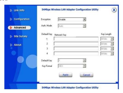
Additional security can be achieved by using the WEP (Wired Equivalent Privacy) encryption. WEP encrypts each frame transmitted from the radio using one of the keys entered from this panel.
