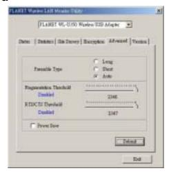
There are **Preamble Type**, **Fragmentation Threshold**, and **RTS/CTS Threshold** settings under this mode.
