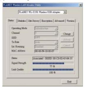
This utility can be used to change the following configuration parameters when the device is active.
