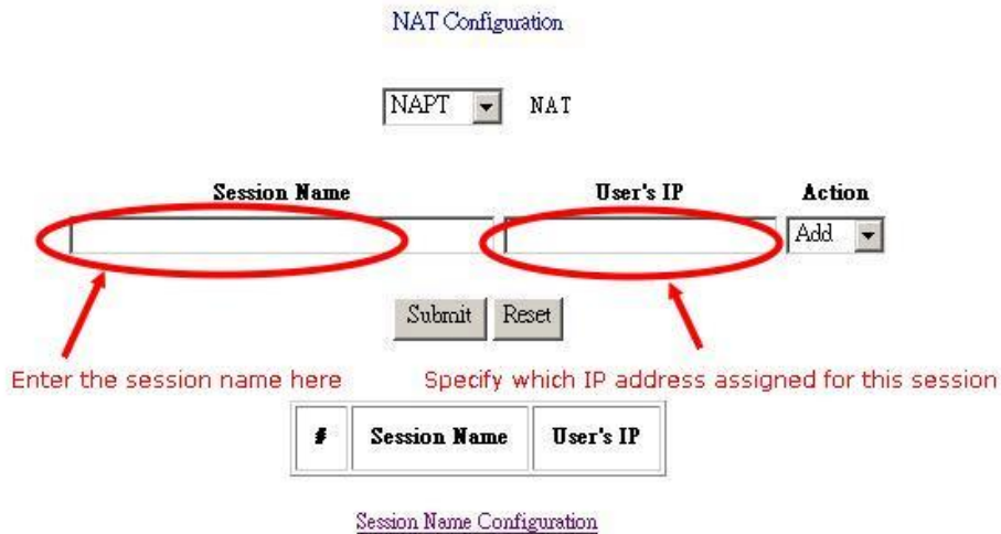
Figure 4-18: NAPT configuration screen
