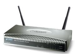
The PLANET WNRT-625 Wireless Router is a built-in 802.11n draft 2.0 access point (AP) device also backward compatible with 802.11b/g. The wireless router features radio in 1x2 (TX/RX) of intelligent antennas offering high performance and enhances superior coverage range.
