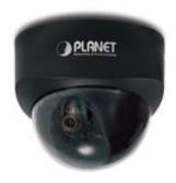
Simultaneously provides MPEG-4 and M-JPEG video streaming, the PLANET ICA-510 is a Dual Mode CCD Dome Internet Camera which uses high resolution 1/3-inch CCD sensor for capturing color images. Equipped with network and analog video output interfaces make the ICA-510 a flexible viewing and recording implementation.
