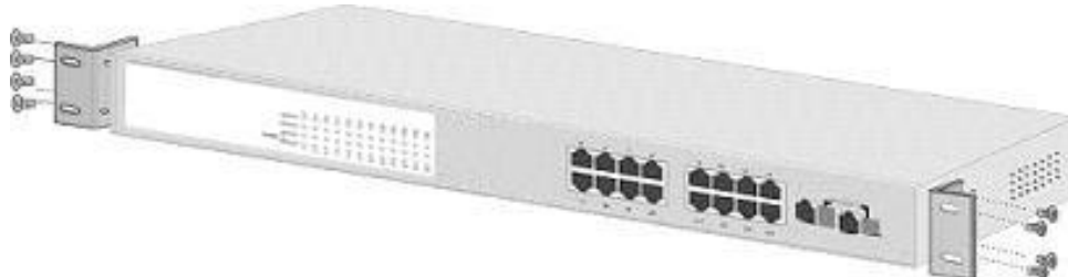
Figure 2-4 Attaching the brackets to the Web Smart PoE Switch
