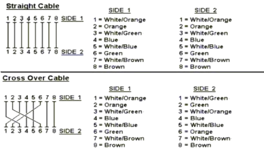
Figure A-1: Straight-Through and Crossover Cable
