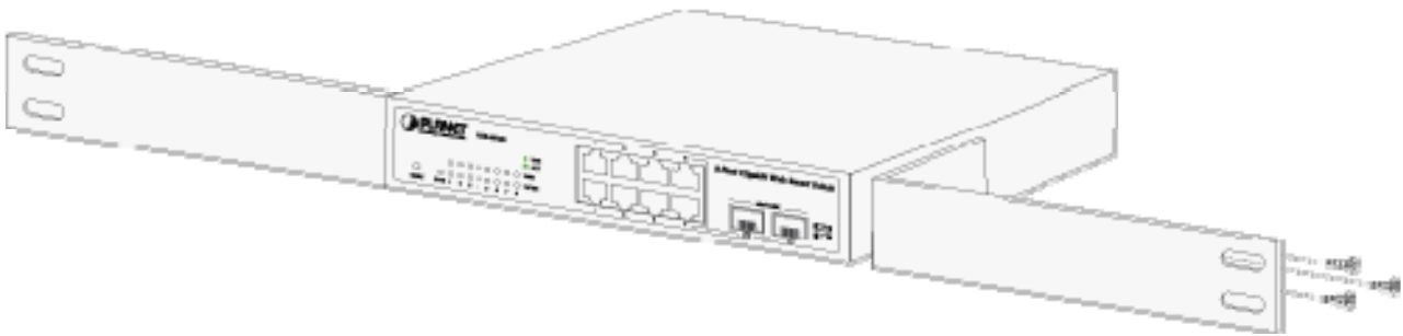
Figure 2-8 Attach brackets to the Gigabit Ethernet Switch.
