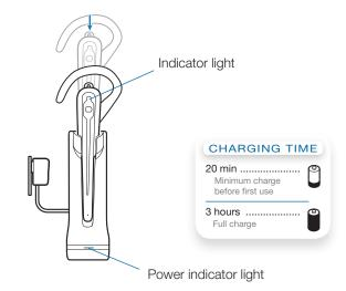
**NOTE** The USB charging cable can also be used to charge the headset. To successfully charge your headset with the USB cable, the PC must be on and in an active state (not standby). The charging time will vary according to the number of other devices drawing power from the PC's USB port(s).
