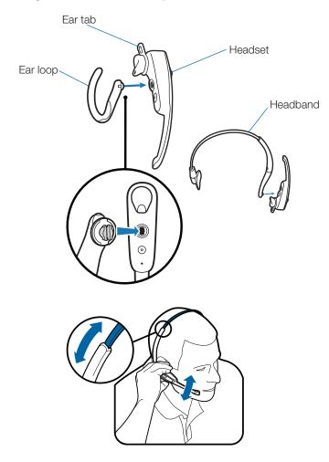
6 The ear tab has been designed to maximise stability of the headset. It can be rotated on the headset to optimise its fit and comfort in the ear. If desired, the ear tab can be removed by pulling the tab from the headset.
