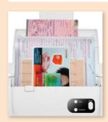
The SmartOffice PS340S is designed to scan business documents up to 50" long and rigid cards, such as ID cards and drivers licenses, up to 1.2mm thick, without operator adjustments. Mixed batches of documents can be scanned without sorting thanks to the class leading paper handling and image processing.
