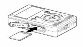
When inserting a memory card in the unit, be careful and insert the card properly as shown in the diagram (taking note of the correct side up) or you may damage the card and/or Ext card slot.
