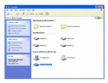
When you connect the unit to a USB port, it will be recognized as a "Removable Disk" in Win XP, 2000, ME
