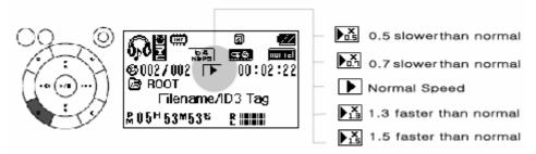
You can change the playback speed of a file by pressing the "SPEED" button. Each press will speed up or slow down the file as follows: x13, x15, x05, x07 and back to normal. This function only works with MP3 files.
