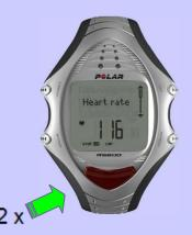
The stopwatch starts, a heart symbol blinks and the horse's heart rate is displayed in the bottom of the screen. From now on, the RS800CX is recording your exercise.
