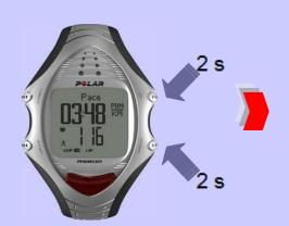
Press and hold **UP** for 2 seconds to zoom in the data of the top row, or **DOWN** for 2 seconds to zoom in the data of the bottom row. Press and hold the same button for 2 seconds to zoom out.
