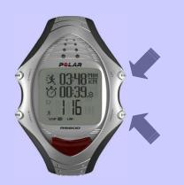
To check the data you are most interested in, change display by pressing **UP** or **DOWN**. (6 different displays are set by default but can be customized – see user manual)
